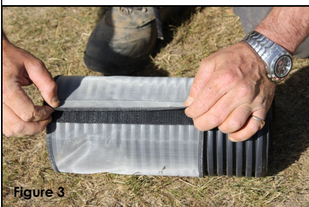
Figure 3. To reinstall screen, wrap tightly around top of bucket so that both holes are covered and Velcro™ fastener is not over holes.
